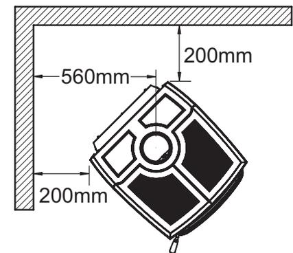
Figure 4. ALT5 AS - SW Shield\_clearances.
