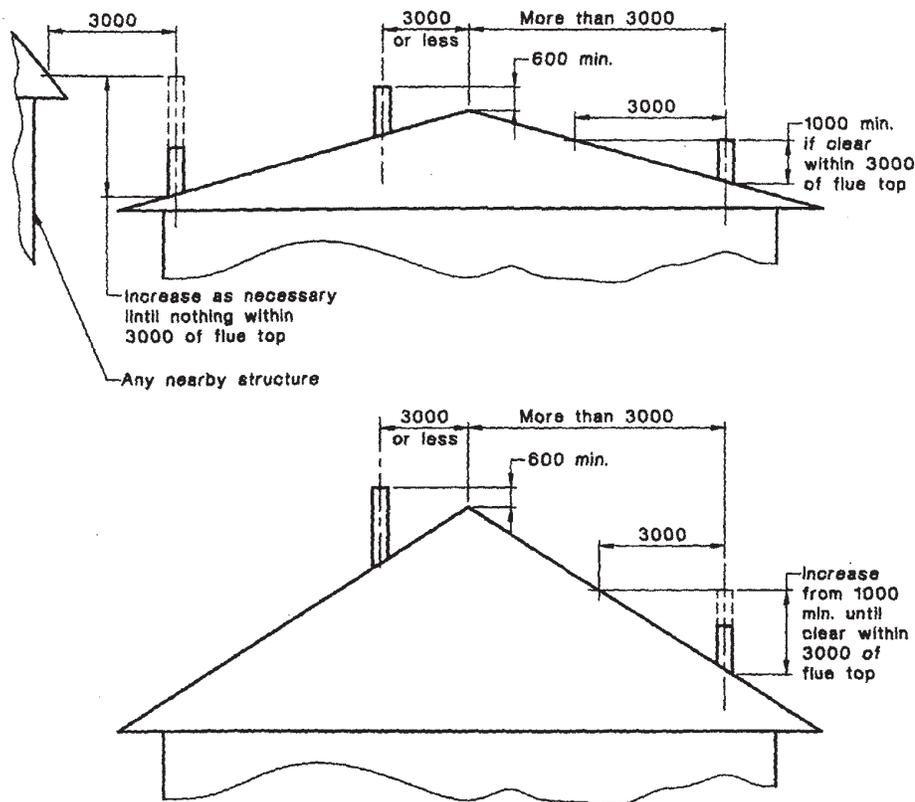
Figure 6. vent termination clearances metric.
