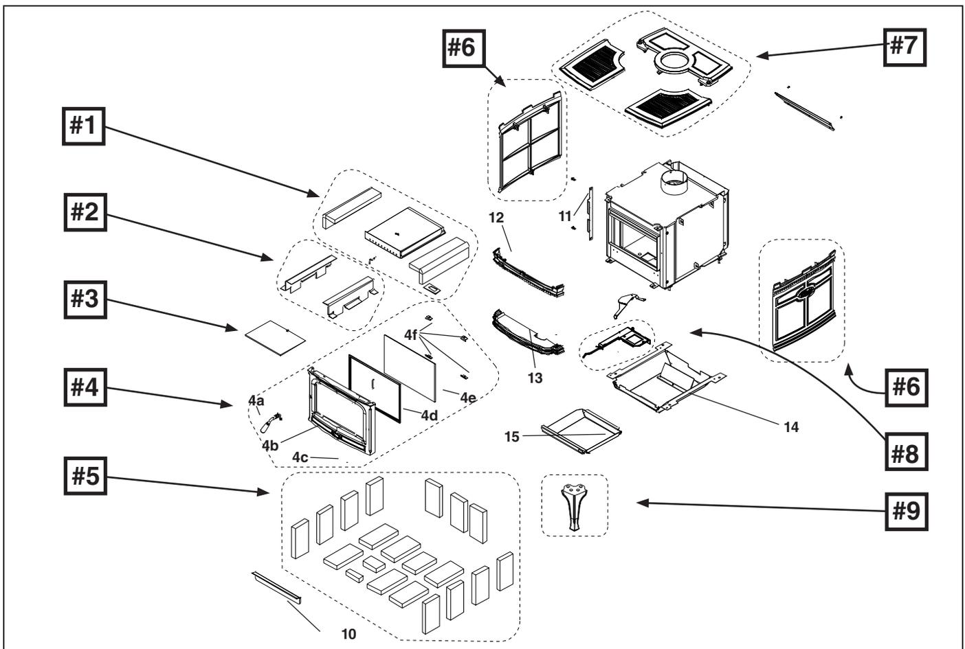
Figure 9. ALT5 AS Exploded View.
