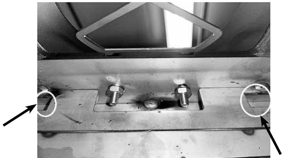
Figure 5. Front mounting slots for Flue Gas Agitator.
