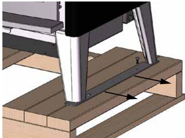
Figure 2. AB25 Hold down removal1.
