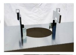
The brackets are fixed to the 8" inner casing is sealed into the top of the Zero Clerance box. And the the upper folded U-shaped hook is fixed to the 10" outer casing to keep it spaced 70mm off the ZCB. These can be fixed with self-tapping screws or rivets.
