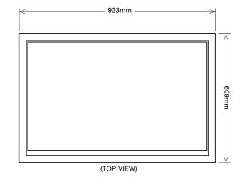
This drop-in BBQ is designed to sit flush with the bench. However, if you choose to install the BBQ on top of the stone bench, you need to make sure the legs are supporting the BBQ.
