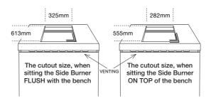
This drop-in BBQ is designed to sit flush with the bench. However, if you choose to install the BBQ on top of the bench, you need to make sure the legs are supporting the BBQ.
