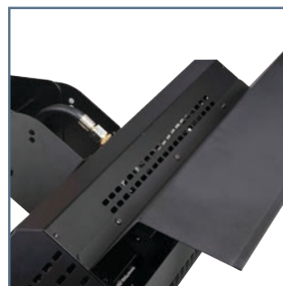
The standard heat reflector ensures only 500mm overhead clearance is required. The optional HeatShield (TGHAC-003) reduces this to 300mm clearance.
