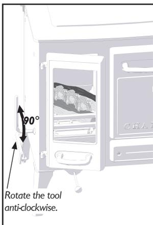
Put the grate into the open position by rotating the tool anti-clockwise. Place 2 small, dry, well seasoned logs into the bottom of the firebox running from front to back. Keep air control fully out and door cracked open.
