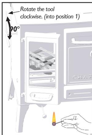
Open the flue gas diverter by pulling the tool forward. Build a stack of 6-8 softwood kindling sticks. This can be in grid shape or a pyramid with paper or firelighter in the centre, ensure to leave a space between the pieces to allow the air to circulate around and through them and light.
