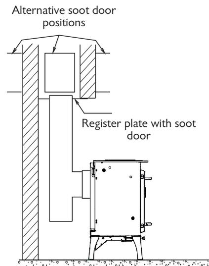
**Fig. 7 Horizontal Register Plate With Top Flue Connection**
