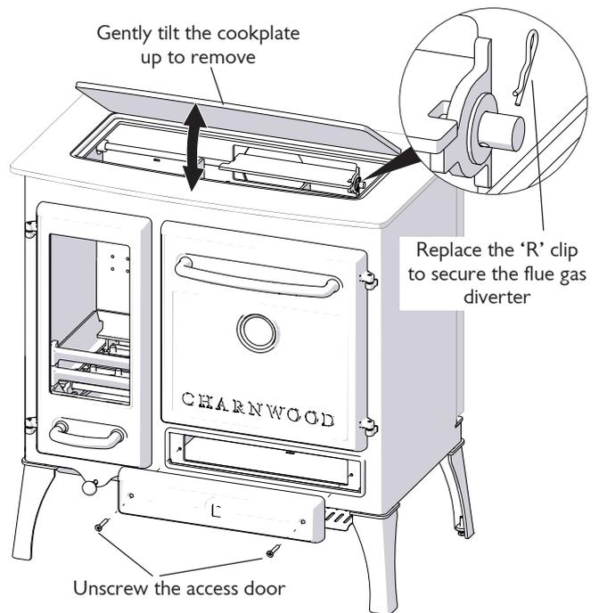
**Fig.5 Cook plate, flue gas diverter and access door removal**
