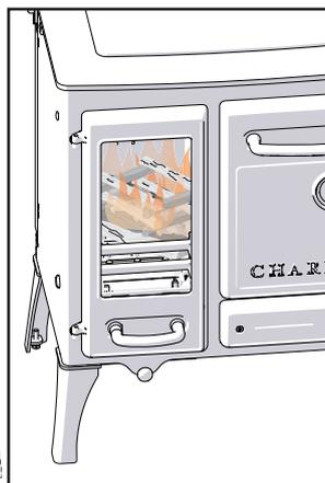
Add larger logs once fire is established. The air control can be reduced to the nominal click position. If cracked open, the door can now be closed. Set the flue diverter into the normal position 2 (push back).
