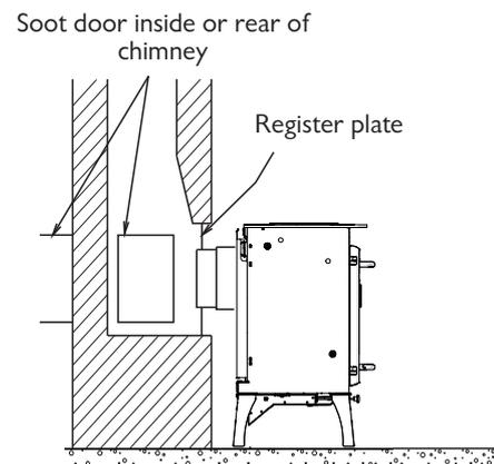
**Fig. 6 Horizontal Register Plate With Rear Flue Connection**
