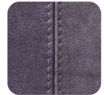
Colour variation occurs during the dyeing process as different parts of the hide absorbs the dye in varying amounts
