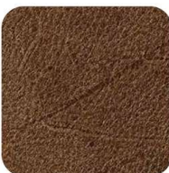
Recovered scar marks causes grain line to be faint
