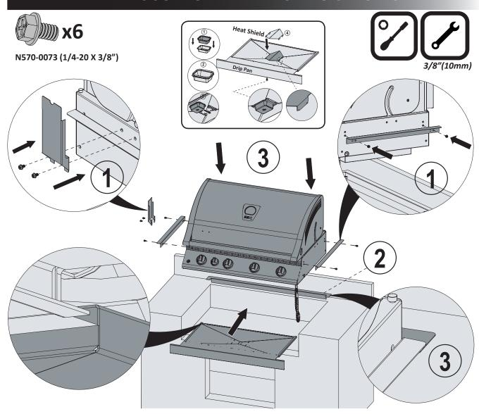
This grill is designed for masonry, **NON-COMBUSTIBLE** enclosures only and must be installed and serviced by a qualified installer to local codes.
