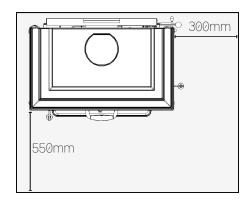
**HEARTH WIDTH:** Due to the side opening door on the Isotto Evo there must be a minimum of 300mm hearth clearance to the right of the fireplace.
